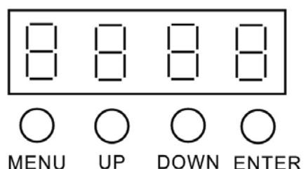
Once your changes are made, press the ENTER button, and then press and hold the MENU button for at least three seconds to confirm and lock the change into the system memory. To exit without making any adjustments, press the MENU BUTTON. The display will lock after 30 seconds. Press the MENU button for 3 seconds to unlock.
